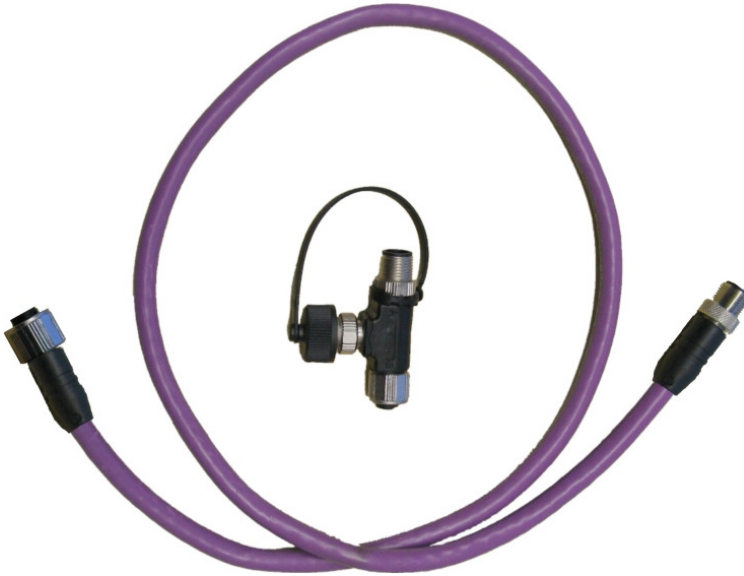
Fig. 6: M12 service interface for testing a live bus
